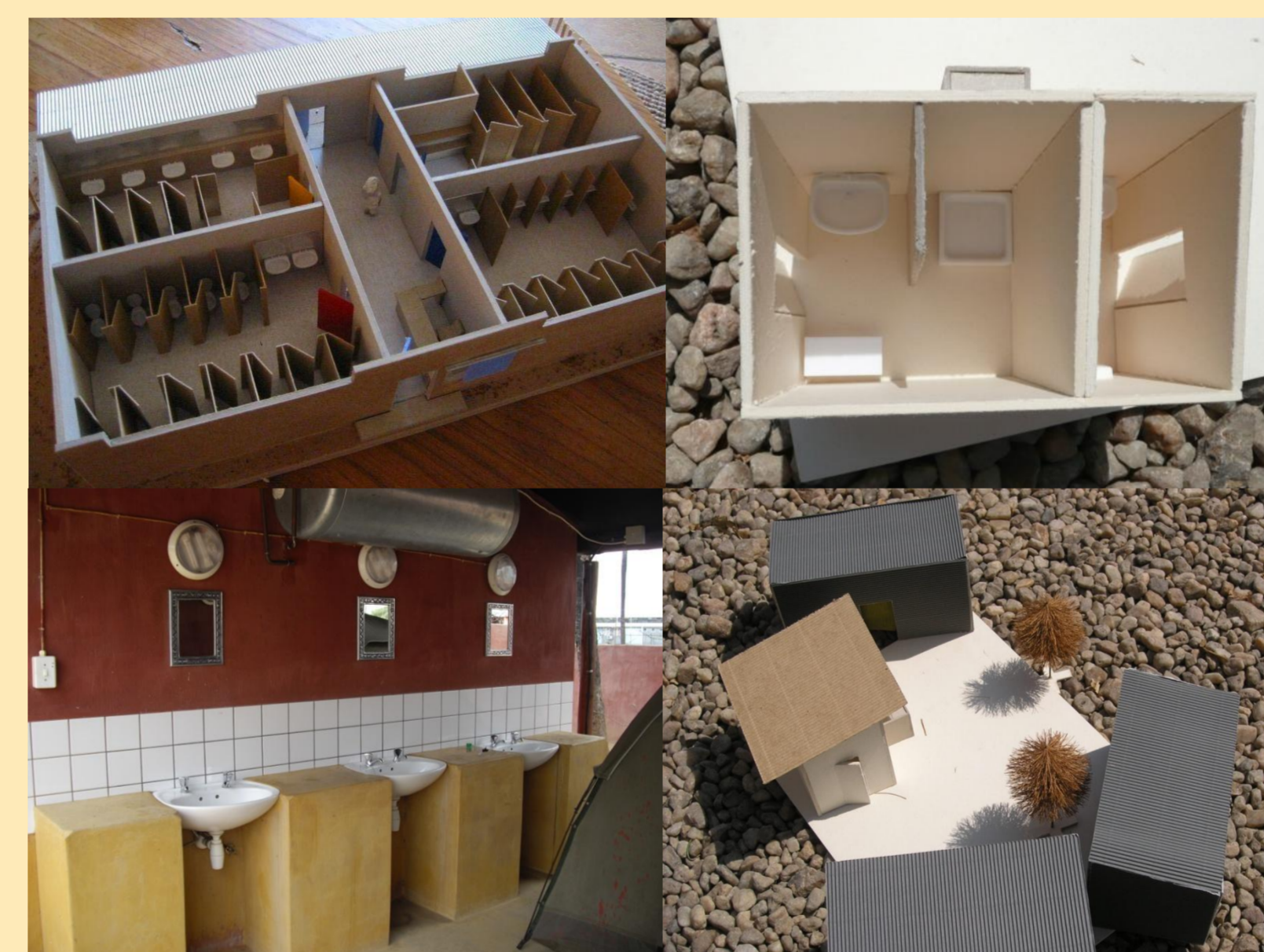
Figure 3: Model and example of a communal washing house (left). Cluster washing house as a model – insight view (upper right), model situation with shacks in the surrounding (lower right). (Deffner, Müller)
